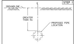
G. TRENCH CONDITION IS WHEN GROUNDLINE ELEVATION IS GREATER THAN HO ABOVE TOP OF PROPOSED PIPE.
