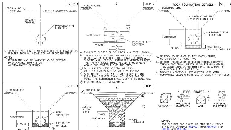
COMPACT BEDDING IN SUBTRENCH IN LAYERS 6" OR LESS TO WIDTH AND ELEVATION SHOWN. LESS TO WIDTH AND ELEVATION SHOWN. EXCAVATE A GROOVE IN THE COMPACTED BEDDING TO CONFORM TO THE OUTSIDE OF THE PIPE. AFTER EXCAVATION OF THE GROOVE, APPROXIMATELY 4" OF BEDDING SHOULD REMAIN BELOW THE OUTSIDE INVERT OF THE PIPE. THE CRADLE SHALL BE GAGED FOR SHAPE AND SLOPE BY STRIKING OR DRAWING A TEMPLATE THROUGH THE GROOVE IMMEDIATELY BEFORE PLACING EACH SECTION OF PIPE.
